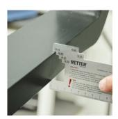
By using the ForkWearMeasuringCard, you can easily decide whether a fork needs to be replaced or not.
