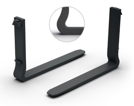
There are goods that could be damaged by the inner heel radius of a standard fork (i.e. wood plates, sensitive pallets etc.). **The solution is swan-neck forks:** The inner heel radius will be relocated backwards. Thus, the nominal length of the fork can be completely used resulting in an increase of safety and efficiency.
