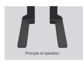
The characteristic feature of cranked forks is the angled shape of the fork back. This special design allows to expand or reduce the spacing between the forks and provides an unobstructed view of the fork tips at the same time. This results in significant benefits in terms of efficiency and safety.
