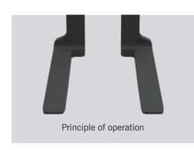
The characteristic feature of cranked forks is the angled shape of the fork back. This special design allows to expand or reduce the spacing between the forks and provides an unobstructed view of the fork tips at the same time. This results in significant benefits in terms of efficiency and safety.
