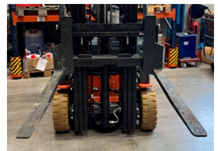
Positioning the fork blade outside the fork carriage
