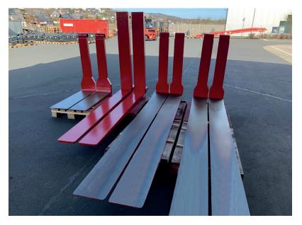
Another highlight is that the fork back is waisted on both sides to provide the forklift driver with a better view of the fork tips, which makes threading between the packages much easier. **The VQ32+ and VQ1300** steel developed by VETTER are perfectly designed for the high, dynamic stresses in the timber industry and ensure 3-fold safety.
