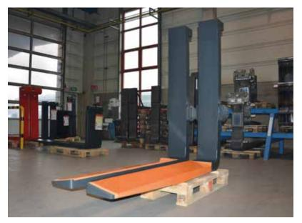
In addition, the fork blades are surfaced with **CROC**<sup>®</sup> coating. This coating prevents the coils from slipping off when braking. In addition, the sensitive surface of the **aluminium is protected and scratches are avoided**.
