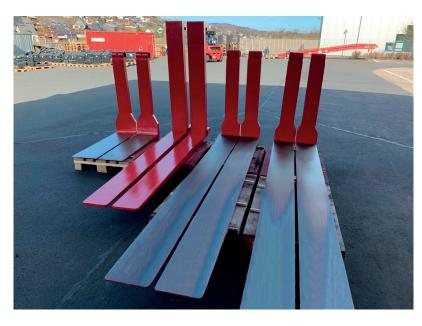
Another highlight is that the fork back is waisted on both sides to provide the forklift driver with a better view of the fork tips, which makes threading between the packages much easier. **The VQ32+ and VQ1300** steel developed by VETTER are perfectly designed for the high, dynamic stresses in the timber industry and ensure 3-fold safety.
