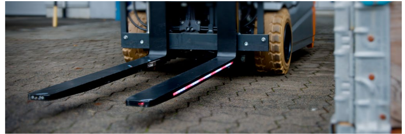
LEDs sideways integrated in the fork blade. Warning function in cluttered situations.
