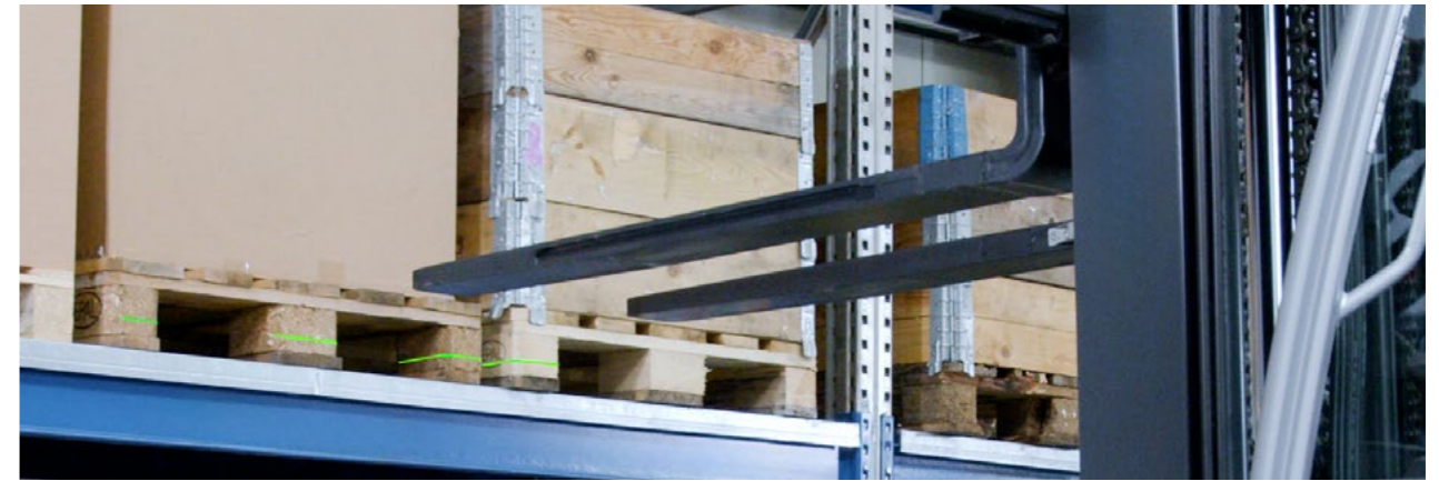
Precise targeting. Green Laser in the fork tip.
