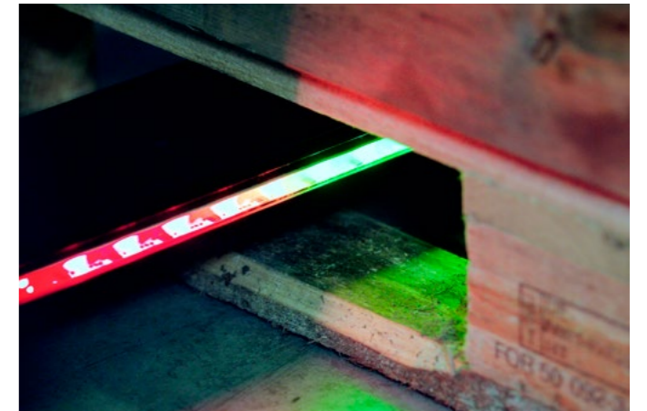
LEDs inside the fork blade. Freely programmable for determining the entry depth.
