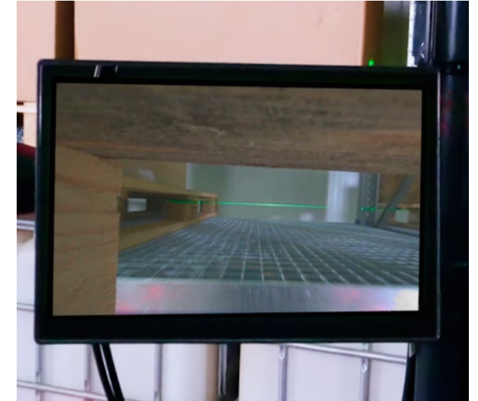
Monitor view FrontCam. View ahead the load.
