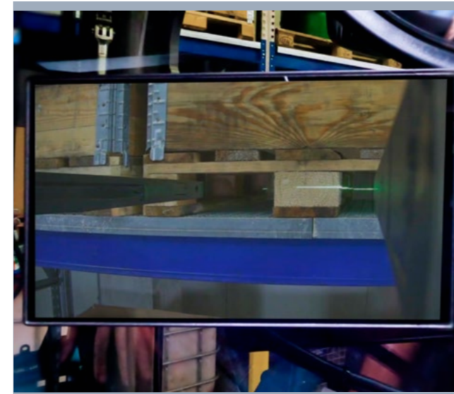
Monitor view SideCam. Targeting at the load carriers along the forks.
