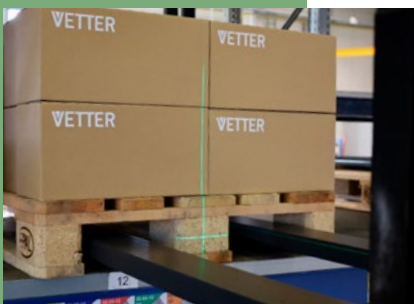
Precise targeting by using the cross laser
