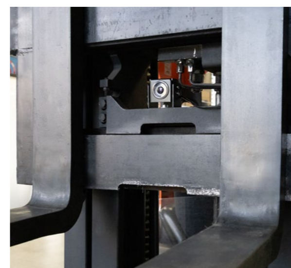
Simple mounting on the fork carrier
