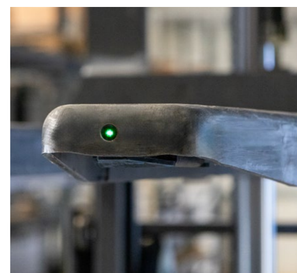
Laser module mounted in the fork...
