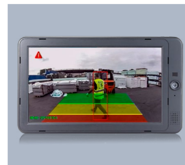
... Person behind the forklift is identified by camera
