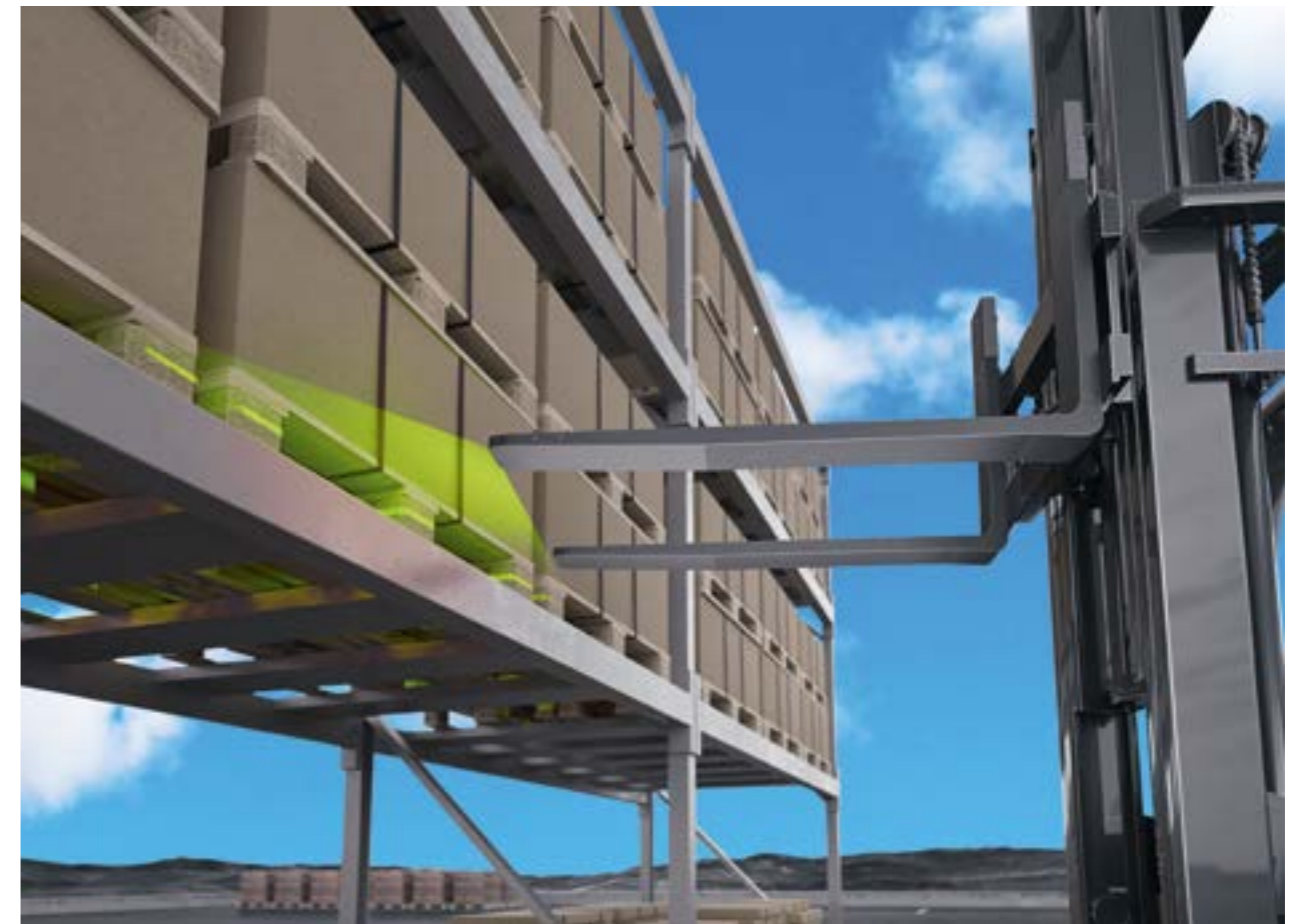
Precise targeting. Green Laser in the fork tip.
