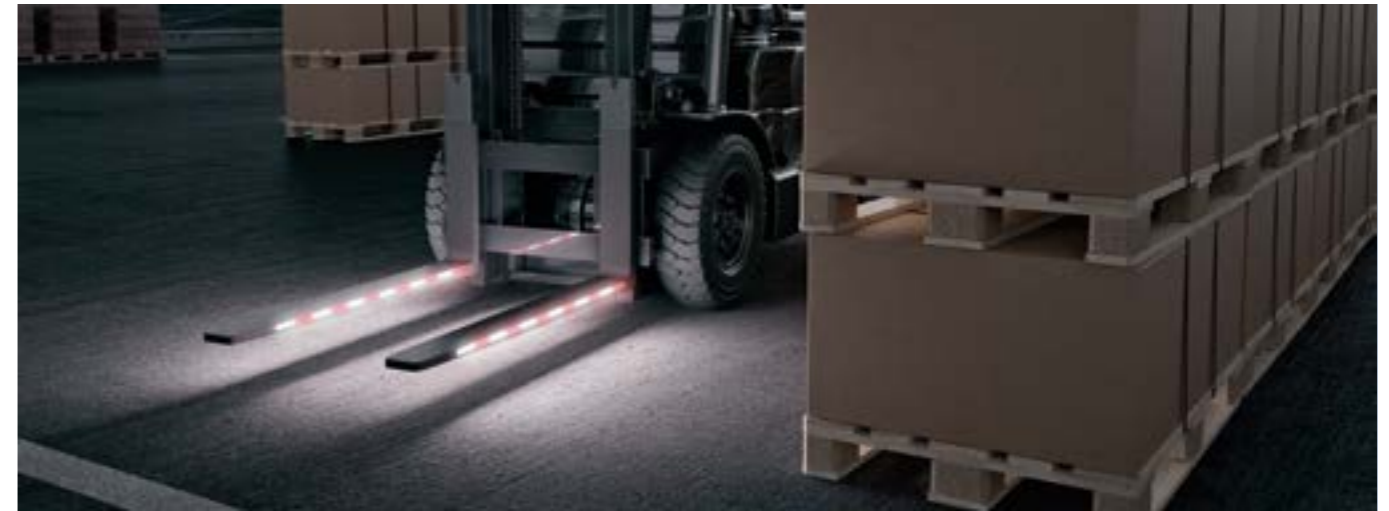
LEDs sideways integrated in the fork blade. Warning function in cluttered situations.
