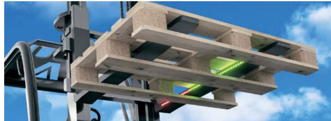
LEDs inside the fork blade. Freely programmable for determining the entry depth.
