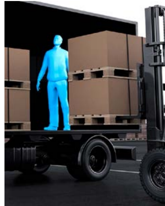
Situation truck loading. Using FrontCam to see people in front of the load.
