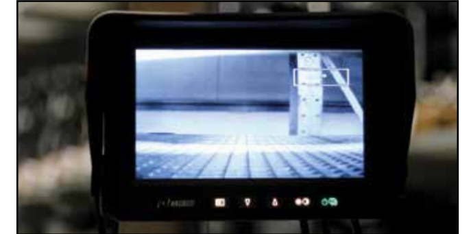
Driver's visibility on the monitor when storing goods with SmartFork® FrontCam
