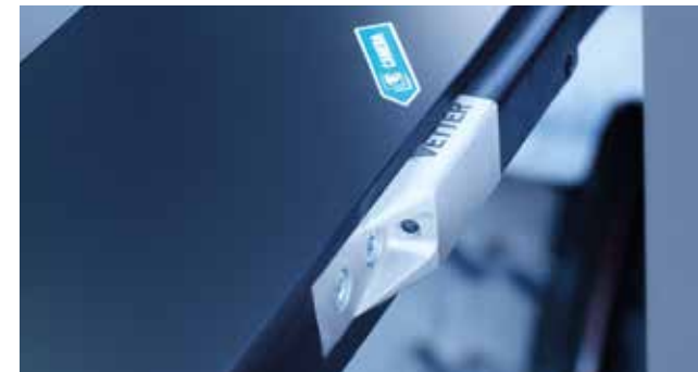
SmartFork® SideCam – partially integrated installation
