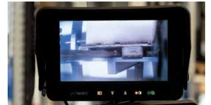
SmartFork® SideCam: monitor during pallet pick-up
