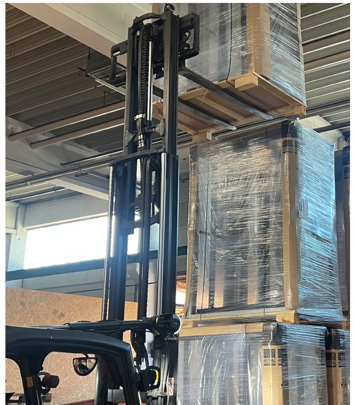
LIZZARD Cam: Camera assistance system for safe pick-up of load carriers.
