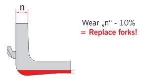
Extract from ISO 5057: "If 10 % of the original fork thickness is worn, the fork has to be taken out of service." 10 % wear of the fork thickness already means a reduction of fork capacity by 20 %. Basis for wear measuring is the original nominal thickness (n) of the fork (f.ex. nominal thickness (n) = 40 mm -> wear limit = 36 mm). Worn forks must not be welded.
