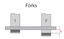
Height difference of fork tips should not exceed  $1.5\ \%$  of the length of fork blade (L).
