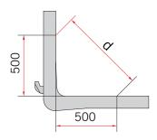
Forks are delivered with an angle of 90°. They are designed with a safety factor 3. i.e. a one-time triple nominal load does not lead to a permanent deflection.
