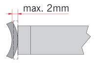
Lateral forces and long-term use may cause lateral bending of fork hook. In this case, fork hooks or forks need to be replaced.
