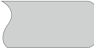
Standard tip for fork widths from 200 mm
