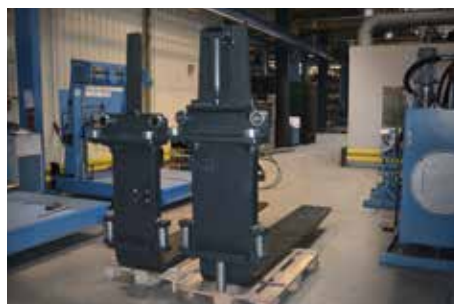
Forks 15¾" x 3¼", roller-guided and height-adjustable
